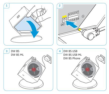
Disconnecting the base station from the mains power supply
