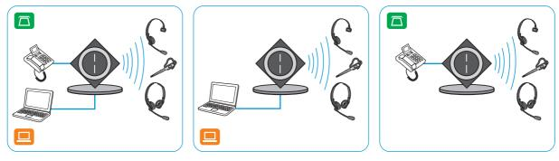
Place the base station at a minimum distance of 15 cm from the fixed line phone.
