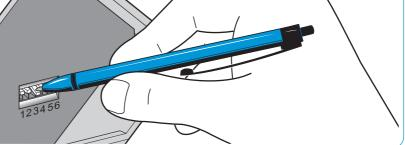
Configuring the handset lifter/hook switch – DIP switches 1 and 2
