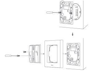
Attach the switch plate to the switching unit.
