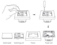
2.Use a screwdriver to loosen the screws on the terminals, connect the live wire to the L hole, connect the neutral wire to the N hole (depending on whether there is a neutral wire in the household wiring), connect the load (light) wire to the L1 hole, confirm the correct wiring, and tighten the screw on the terminal.
