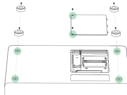
3. Turn to the back of the device, then remove the screws that secure the back ventilation cover.
