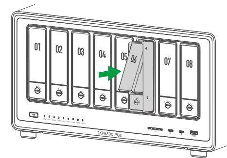
! For installing 3.5-inch hard drives, please remember to move the fastening pin back to the rear end.
