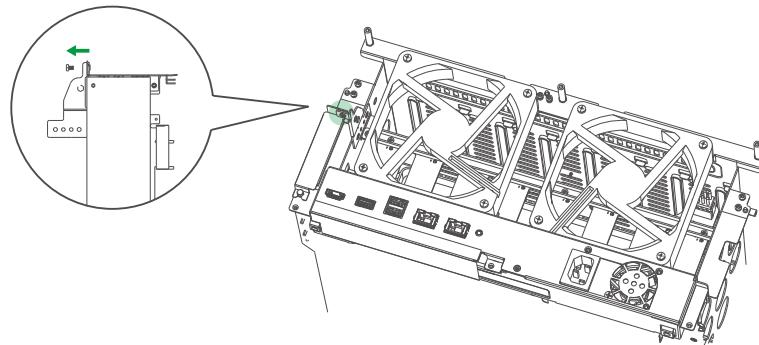
6. Insert the card into the slot and ensure the card is connected securely, then tighten the screws.
