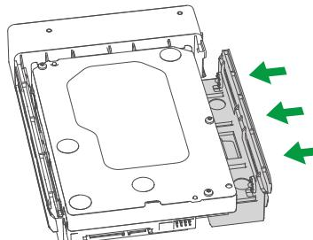
5. Load the tray into the bay: Insert the loaded drive tray into the empty drive bay and lock it.
