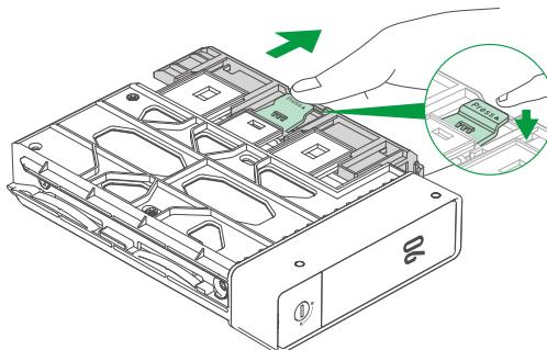
3. Install the drive: Place drive on the tray. Ensure the four fastening pins on the tray (two on each side) are aligned with the screw holes on the drive.
