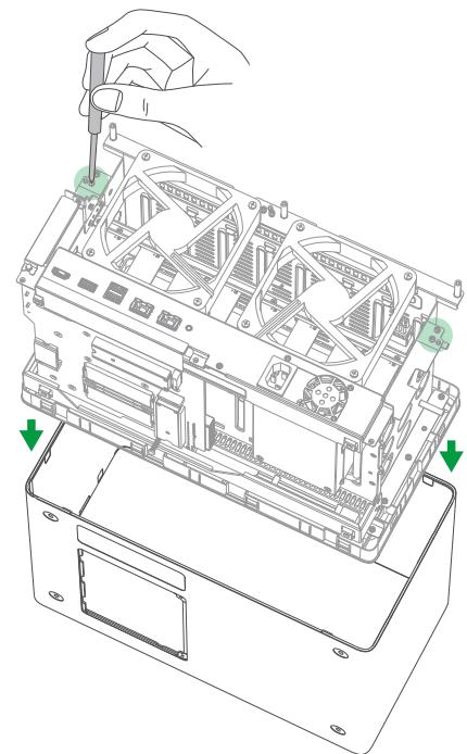
5. Remove the screw on the existing bracket. Then remove the bracket and keep it in case you need to replace the PCIe expansion card.
