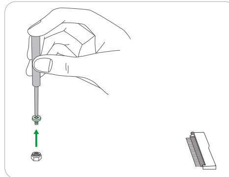
3. Insert M.2 SSD into the slot in the direction as shown in the image, then tighten the screws.
