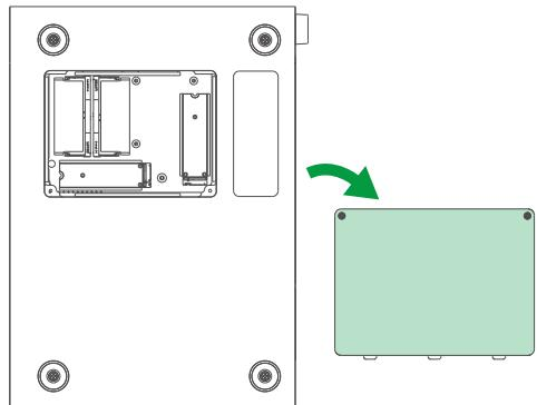
2. Unscrew the M.2 fixing screws.
