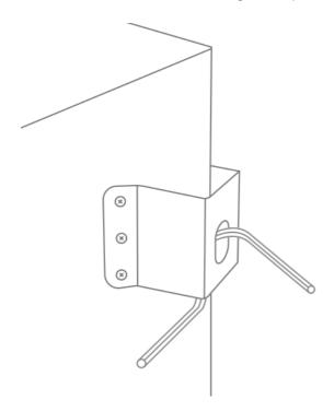
Then, screw the camera to the bracket according to the holes and adjust the camera angle for the best coverage.
