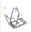
Close the bracket that holds the CPU. Close the retention cover and fasten the screw .
