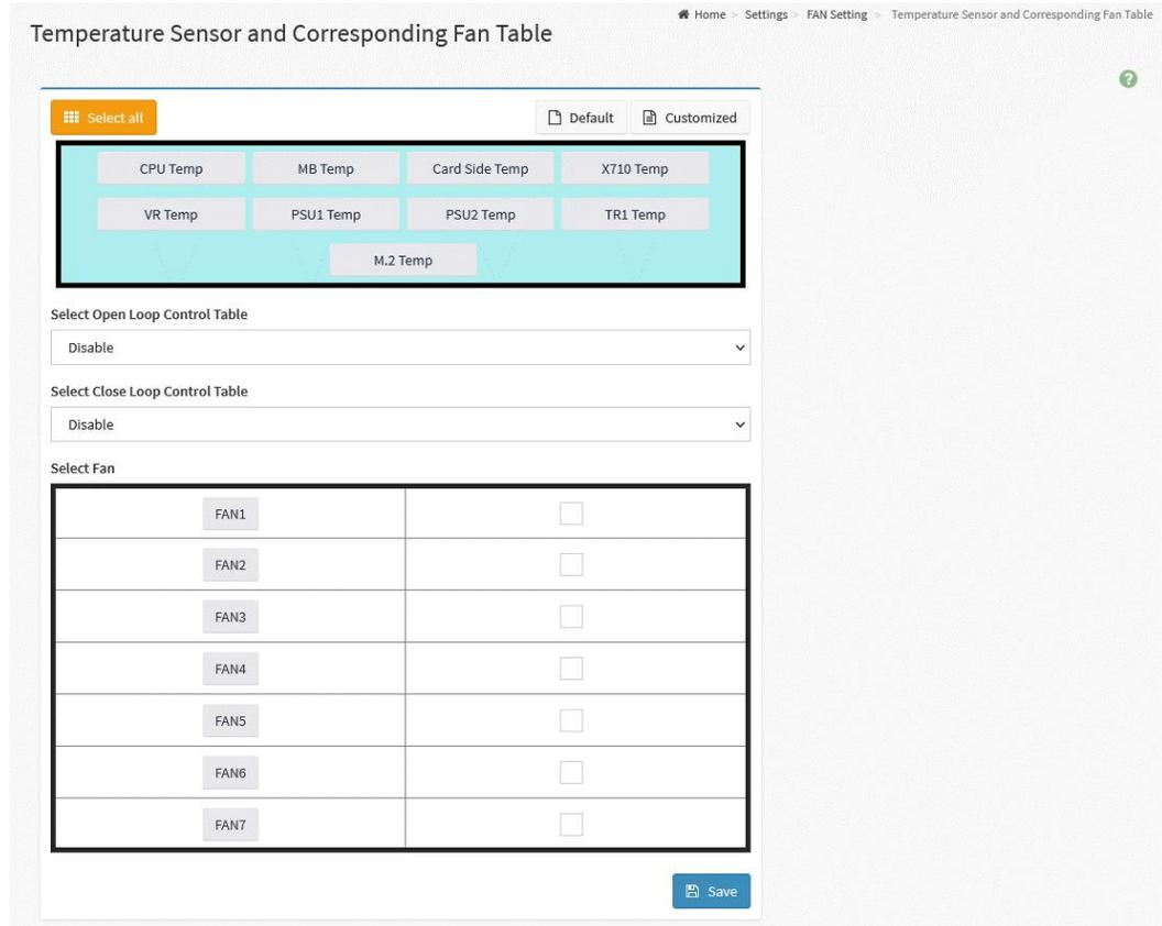
**Figure 105. Temperature Sensor and Corresponding Fan Table Page**
