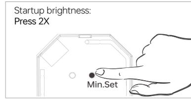
Short press the button twice to set startup brightness: when current brightness value is 1%-50%, it will be set as startup brightness. When current brightness value is 0%, previously set startup brightness will be deleted.
