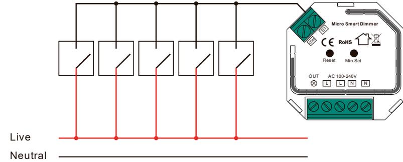
This phase dimmer adopts leading edge dimming (forward phase control) or trailing edge dimming (reverse phase control), two versions are available for choosing, factory default version is trailing edge. Please make sure the connected loads support the control type you choose. Please refer to the user manual of the load or consult the supplier of the load.
