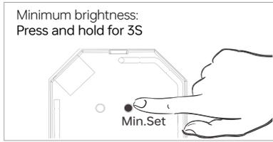
Press and hold down the button for 3 seconds to set minimum brightness: when current brightness value is 1%-50%, it will be set as minimum brightness. When current brightness value is 100%, previously set minimum brightness will be deleted. Once a minimum brightness is set, the connected load can not be dimmed below this level.
