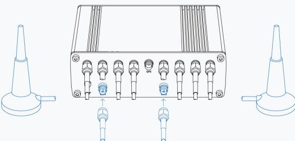
**8. Attach the GPS antenna to the connector labeled "GPS".**
