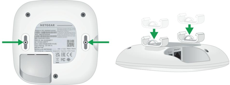
1. Use the two provided small screws to attach the T-bar hooks to the AP
