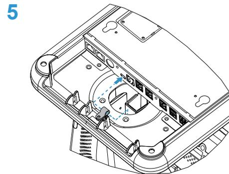
Plug in the other end of the USB-C cable to the base and secure with the supplied cable clamp and screw from bag C.
