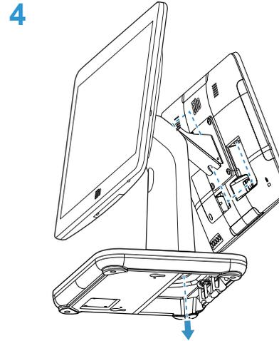
Attach a monitor to the display bracket using (4) screws from bag B. Plug in the USB-C cable and route through the stand.
