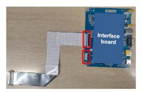
Assemble "Interface board" to "Main Shielding"
