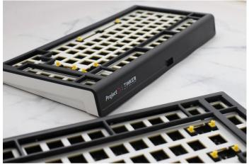
the baseplate is manufactured from FR-4, a laminate-grade glass epoxy. It is a versatile thermoset plastic that has a high stiffness to weight ratio. A rubber gasket is utilised for mounting switches. To cushion the switches as you type is a layer of Poron foam, providing a dampening effect to soften the click and exceptional typing feel.
