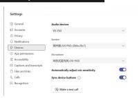
To make sure the setup in correct, open MS Teams > Settings > Devices, you should be able to see the Audio devices, speaker and microphone showing "VX-P60" as the selected driver. If you do not see this, choose "VX-P60" from the drop-down menu.
