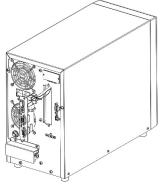
**Step 4:** Install new parallel board with 2 screws tightly. Now the UPS is providing parallel operation function.
