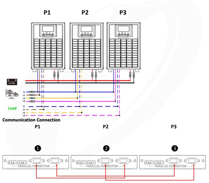
**WARNING:** Do not connect the current sharing cable between the UPS which are in different phases. Otherwise, it may damage the UPS.
