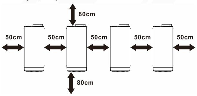
**NOTE:** For proper air circulation to dissipate heat, allow a clearance of approx. 20 cm to the side and approx. 50 cm above and below the unit. Be sure to install each unit in the same level.
