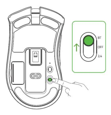
2. Press and hold the two side buttons and the DPI stage up button simultaneously for three seconds to activate pairing mode. The Razer logo will blink twice in repeated intervals to show that the device is in pairing mode.
