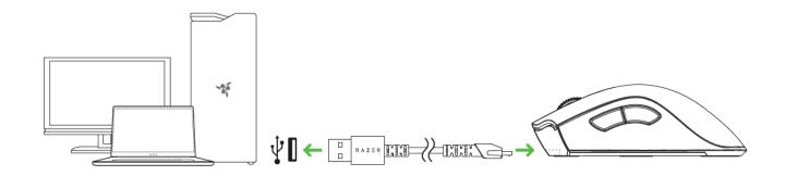
The Razer DeathAdder V2 Pro requires a USB connection that can supply sufficient power to charge the device. The charging process may be affected when connecting to a non-powered USB hub or non-powered USB port mostly found on keyboards and peripherals. It's recommended to always connect the Razer DeathAdder V2 Pro directly to the USB port of your computer.
