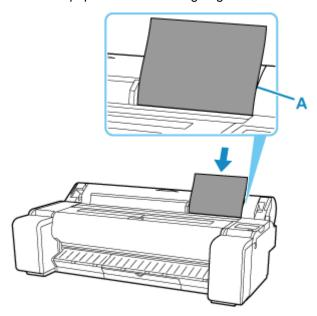
**5.** Move the width guide (A) carefully to match the size of paper loaded.
