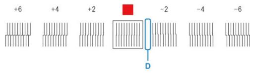
**9.** Open top cover and move angle adjustment lever to match number (or square) of straightest set of lines.
