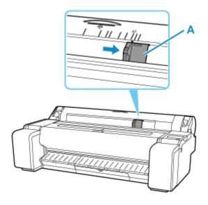
**4.** Load a single sheet printing-side up in the feed slot, with the right edge aligned with the paper alignment line (A) to the right of the roll paper cover.
