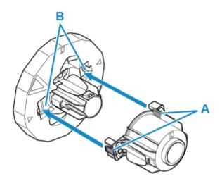
**10.** Insert holder stopper from left into roll holder, and then while holding the end plate (B), push firmly until holder stopper flange (A) touches roll paper.
