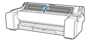
7. Align the angle adjustment lever with the red square and close the top cover.
