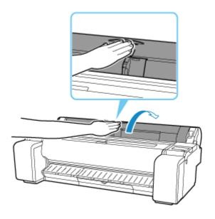
**3.** Using both hands, rotate the roll holder toward the back to rewind the roll.
