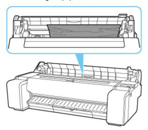
• If the paper is jammed by the ejection guide
