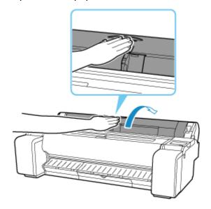
**5.** Place the roll paper in the pocket on the top surface of the printer.
