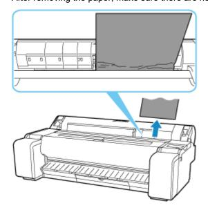
If the paper is jammed by the ejection guide
