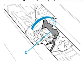
**16.** Align angle adjustment lever with the red square position.
