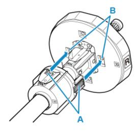
**8.** With leading edge of roll paper facing forward, insert Roll Holder from right side of roll. Insert firmly until roll paper touches flange (A) of roll holder.
