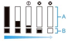
If the touch screen indicates to replace the ink tank, replace the ink tank. If a message is displayed indicating to check the remaining ink levels, or after tasks that consume a lot of ink such as large-format printing or head cleaning, check the remaining levels and replace ink tank as needed.
