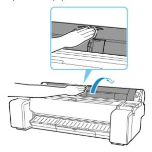
6. Using both hands, rotate the roll holder toward the back to rewind the roll.
