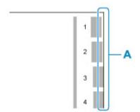
Check the paper edge (A) of the 1st to 8th on the output pattern and select the number that has the appropriate amount of extension.
