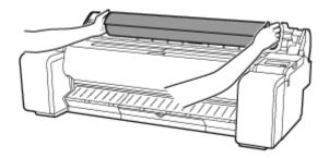
**6.** Rotate the holder stopper lever (A) towards to release the lock, and while holding the end plate (B), remove holder stopper from the roll holder.
