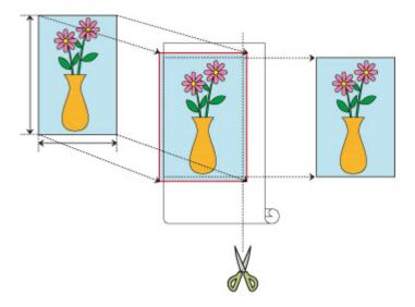
With the three-sided borderless printing feature, you can print with no borders on three sides if the paper sizes don't match the roll paper width.
