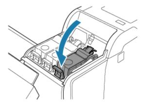
• Do not push the ink tank in by hand. Forcing the ink tank into the holder may damage the printer.
