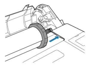
**13.** Holding the roll holder flange (A), guide the holder along the slide guides (B) on both ends, keeping the holder level as you load it in the roll holder slot.
