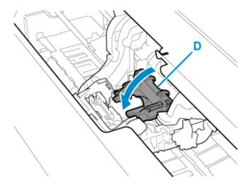
**15.** While holding center part (C) of print head lock lever, lower it toward back.
