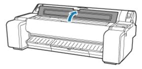
**6.** If the print head locking cover and print head lock lever are dirty, use a damp cloth that you have wrung out completely to wipe them clean.
