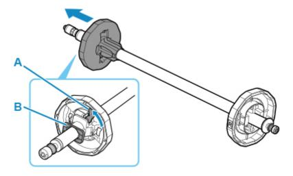
**7.** If using 3-inch core paper, align 3-inch paper core attachment tabs (A) with roll holder holes (B) and insert firmly.
