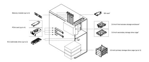
In the 3.5-inch front-access storage enclosure or 3.5-inch storage drive cages, you can install 3.5-inch storage drive or 2.5-inch storage drive with a storage drive converter.
