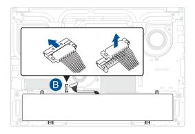
To connect the battery, align and connect the cable to the battery connector before you reattach the compartment cover.
