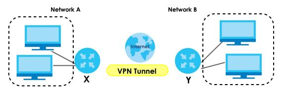
The VPN tunnel connects the Device (X) and the remote IPSec router (Y). These routers then connect the local network (A) and remote network (B).
