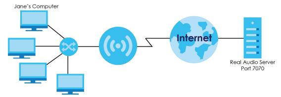
Figure 65 Trigger Port Forwarding Process: Example
