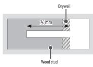
Use the Ø 4 mm drill bit for wood to drill holes with the depth of 76 mm. (Clean the drilled hole.)
