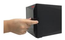
2. Using the latch, gently pull the disk tray out of the disk bay.
