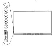
The convenience panel provides buttons for turning the display on and off, controlling the volume, freezing and unfreezing the screen, and showing and hiding a screen shade. It also includes connectors for USB peripherals and a computer or other input source (available connectors vary by model, see Connecting room computers and guest laptops on page 37).
