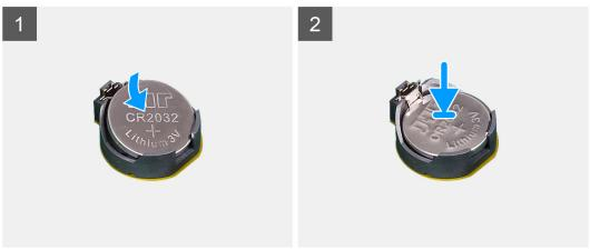
Insert the coin-cell battery into the socket with the positive side (+) label facing up and snap the battery in the socket.
