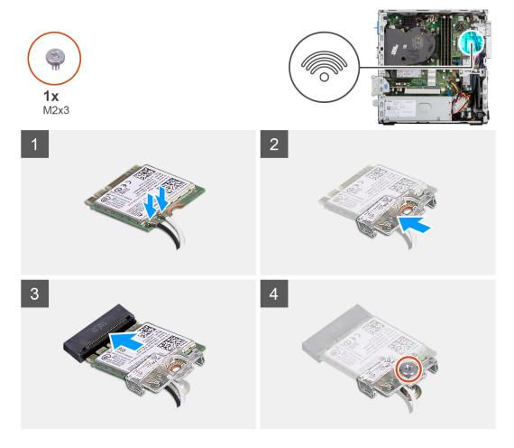
Connect the antenna cables to the WLAN card.
