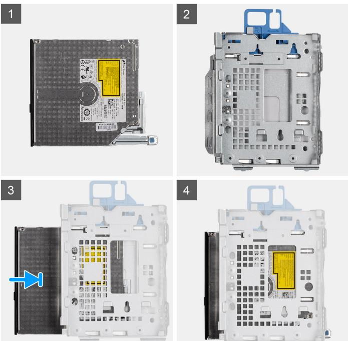
Slide the optical drive into the disk-drive cage until it snaps into place.
