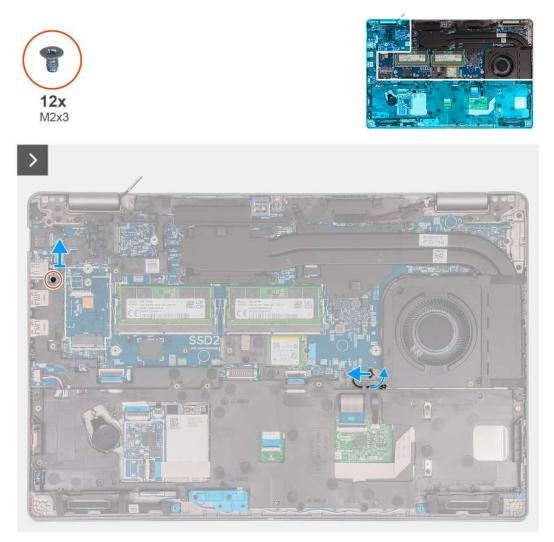
Figure 2. Inner frame removal
