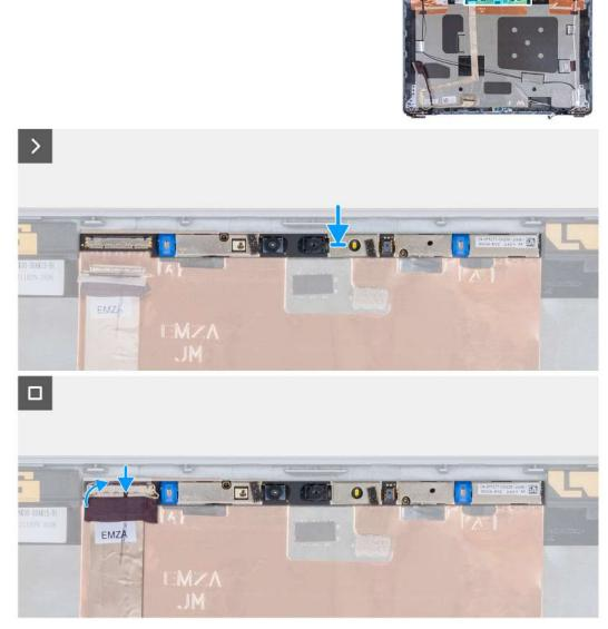
Figure 5. Installing the camera module
