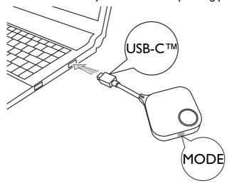
2. When the InstaShow Button is successfully connected to the laptop, the LED indicator of the InstaShow Button will blink red.
