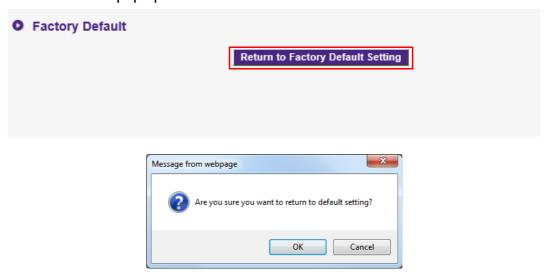
When the process is confirmed the InstaShow Host will begin restoring to **Factory Default** and the LED will quick flash red (flash red twice every second) then restart. After the InstaShow Host restarts the entire process is complete.
