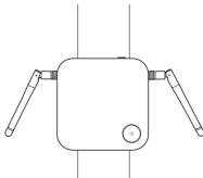
• Avoid positioning the antennas in a horizontal manner, this may result in a weak signal reception:
