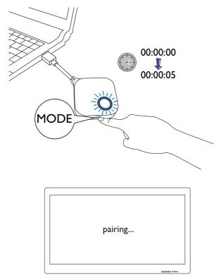
6. The LED indicator of the InstaShow Button will turn static green when the InstaShow Host and InstaShow Button are successfully paired.
