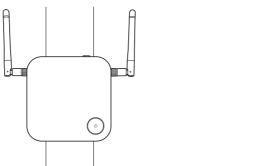
• If you encounter bad signal reception after initial use of the InstaShow Host you can manually adjust the antennas so that they tilt at a slight angle to maximize signal reception. When doing so, avoid tilting the antennas toward the ceiling mount:
