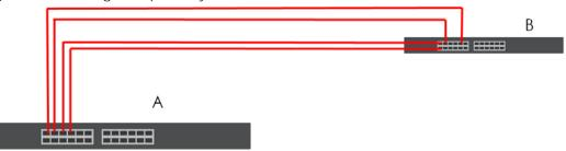
Figure 126 Trunking Example - Physical Connections
